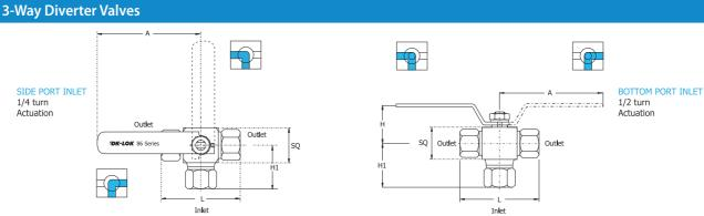
V86 3-way ball valve is designed to switch media through the inlet port and direct it to out of two outlet ports.
