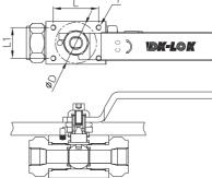
Pad-Lock applicable constructed on upper
